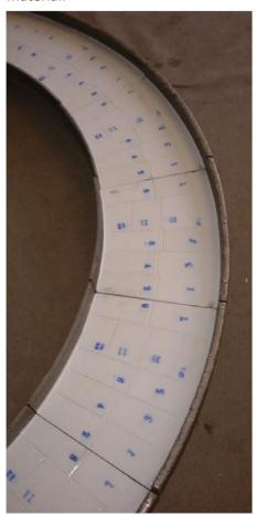
ALDUR® 240 is produced from a complex blend of powders containing 92% alumina (Al203) of outstanding purity.
